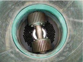
Roller Parts: Rollers are the core parts for making pellets. The rollers of our pellet making machines are made of precise material of alloy metal which makes the roller anti-bearable and no easy to broken. The simplest pellet making machine has one pair of rollers. But now, the new developed flat die pellet maker have two or three pair of rollers which have bigger capacity of making pellets.
