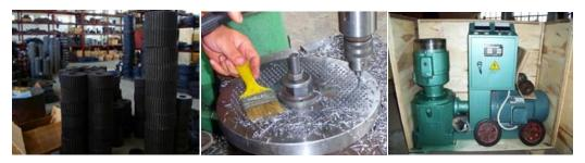
Choose flat die pellet machine for fertilizer or home pellet making can reduce both the production costs and spare parts costs. Moreover, heating treatment can increase the lifespan of flat dies while ring dies buckle under heat treatment and increase pelleting cost. Also it has be proved that pelleting low density raw materials with ring die is inappropriate.
